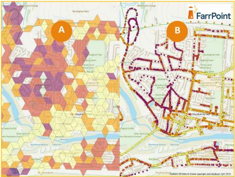
The sample coverage (left) depicts the received signal strength, with lighter shades showing weaker coverage than the darker areas.
